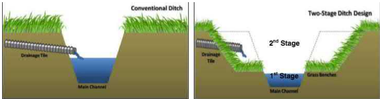
Figure 17. Comparison of conventional and 2-stage ditch.
