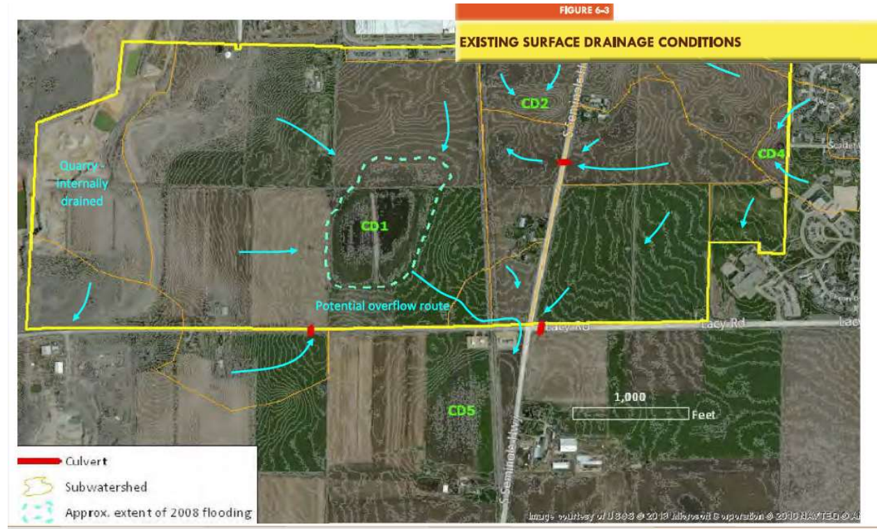
Existing surface drainage conditions with closed depressions (CD)
