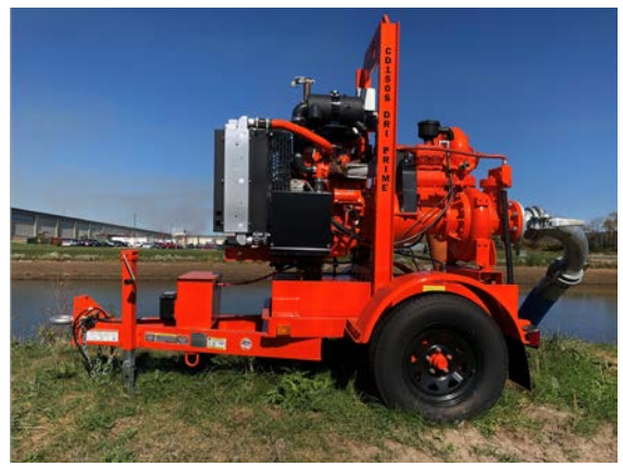
Figure 14 6-Inch Mobile Trailered Pump
